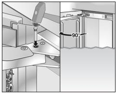
Insert the pin into the hinge from above, as shown.
